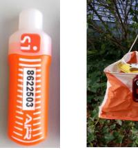
6. For the participants using traditional SI Card, it is required to punch the "Finish" unit when you reach the finish. The timing stops when participants punch the "Finish" unit and the unit will feedback with "beep" sound and flashing optical signal as confirmation.
