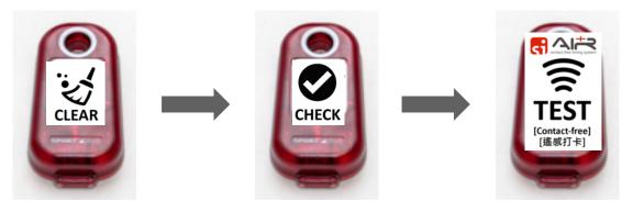
2. SPORTident Air+ is a contactless timing system. The effective range between the control station and the SIAC card is about <u>30 cm (roughly the size of an orienteering flag)</u>. Upon successful "punching", the SIAC card will feedback with flashing optical signal and "beep" sound. If runners cannot find the above signal, they have to return to the control point and do the punching again.
