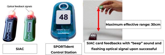
3. If the SIAC card is running low in battery, the contactless punching function will be disabled. If the SIAC card does not feedback with flashing optical signal and "beep" sound even within 30cm
